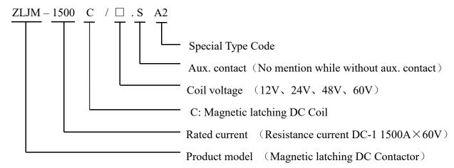
Example: ZLJM-1500A/48.SA2; means: Magnetic latching DC Contactor, 1500A for DC-1 load rated current, coil voltage 48V DC, with aux. contact.
